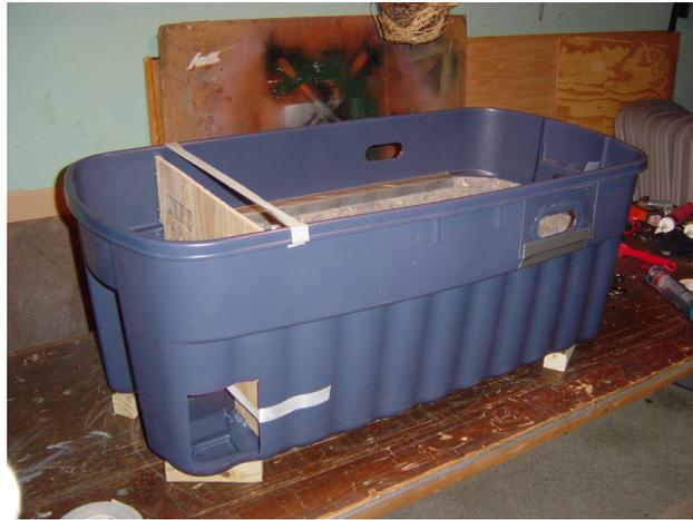
Next you want to glue the partitions into the tubs. Lexal is one of the few tube based sealants that sticks well to these plastic tubs. It’s expensive compared to tub/tile sealant but after all this work you want a strong joint.
